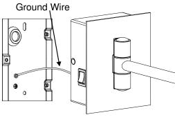
3. Feed the electrical wire from the electrical box, through the mounting plating, and reserved convenient length.
