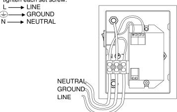
5. Secure the mounting plate to the electrical box on the wall with two (2) wall anchors and mounting screws.
