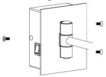
2. Remove the mounting plate from the base, inspect and ensure the terminals of ground wire are tighten on both side.
