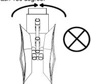
7. DO NOT rotate mirror or arms rapidly or in great force over 20LBS. Correct rotation should be slow and gentle. **DO NOT** rotate mirror in single direction repeatly for many times.
