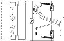
6. Install mirror and wall mount over the wall plate and secure using the three (3) mounting screws.
