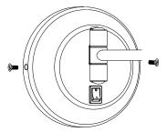
2. Remove the mounting plate from the base, inspect and ensure the terminals of ground wire are tighten on both side.
