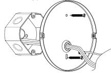
6. Install mirror and wall mount over the wall plate and secure using the two (2) mounting screws.
