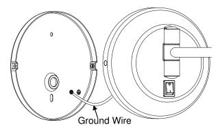
3. Feed the electrical wire from the electrical box, through the mounting plating, and reserved convenient length.
