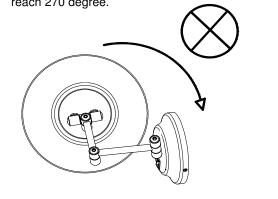
5. **DO NOT** rotate mirror or arms rapidly or in great force over 20LBS. Correct rotation should be slow and gentle. **DO NOT** rotate mirror in single direction repeatly for many times.
