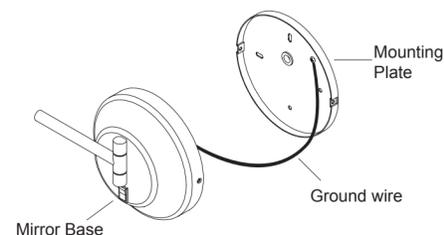
5. Secure the mounting plate to the electrical box on the wall with four(4) wall anchors and mounting screws.
