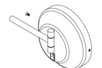
4. Remove the mounting plate from the base.
