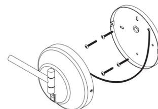
6. Connect the electrical wires coming from the electrical box to the terminal connections. Tighten the set screws.
